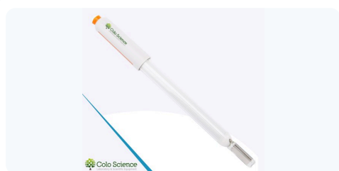
PRO6157 Conductivity electrode DJS-0.1VTG (k = 0.1, ATC) 0.05–200 \mu\text{S/cm} , glass body, with temperature sensor, 0–80 °C, \Phi 12 \times 120 mm; 5-pin connector. Optional
