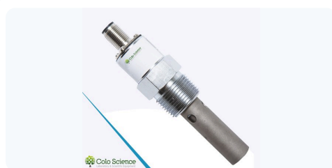
PRO6158 Conductivity electrode DJS-0.01VT (k = 0.01, ATC) 0.05–20 \mu\text{S/cm} , titanium alloy, with temperature sensor, 0–60 °C, \Phi 18 \times 50 mm; 5-pin connector. Optional
