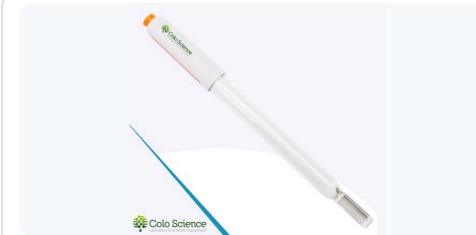
PRO6156 Conductivity electrode DJS-1VTG (k = 1, ATC) 2–3000 \mu\text{S/cm} , glass body, with temperature sensor, 0–80 °C, \Phi 12 \times 120 mm; 5-pin connector. Optional
