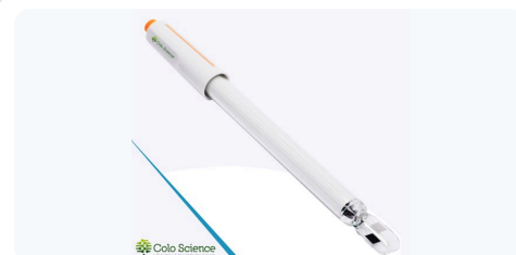
PRO6160 Conductivity electrode DJS-10VTC (k = 10, ATC) 2000–200000 \mu\text{S/cm} , glass body, with temperature sensor, 0–80 °C, \Phi 12 \times 120 mm; 5-pin connector. Optional
