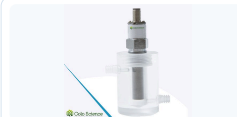
PRO6159 Conductivity electrode DJS-0.01VT (k = 0.01, ATC), flow cell 0.05–20 \mu\text{S/cm} , titanium alloy, with temperature sensor, 0–60 °C, removable flow cell; 5-pin connector. Optional
