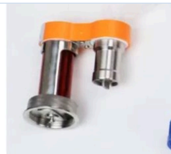
Burette and electrodes • 10 mL burette, platinum, silver and reference electrodes in the standard delivery
