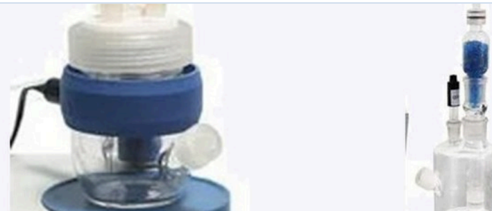
Titration cells • volumetric cell and coulometric generator cell
