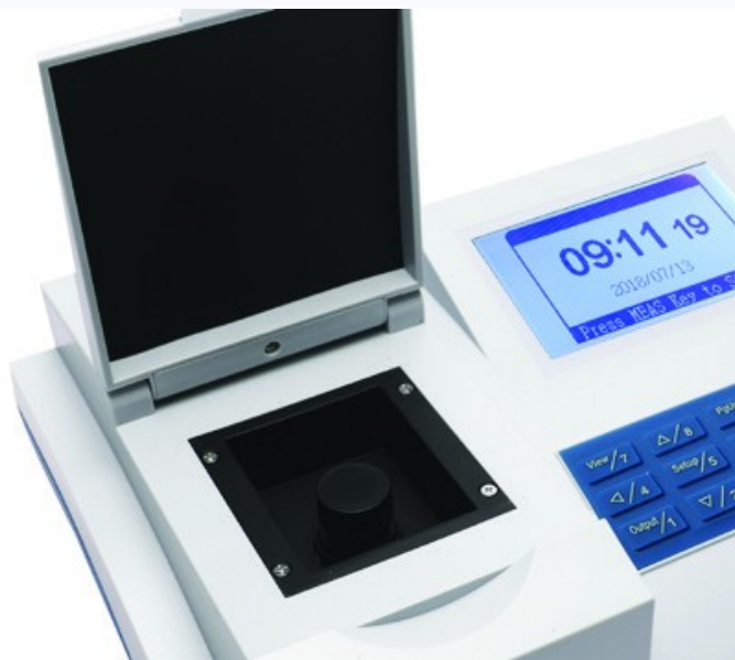
COD100 measuring slot with flip-up lid
