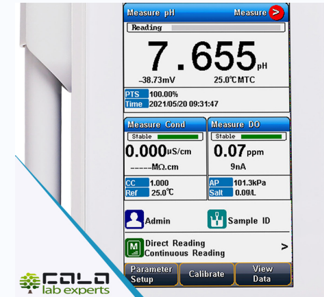
4.3" touchscreen display · method navigation, calibration and measurement control
