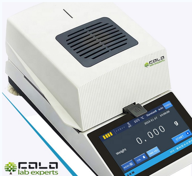
FAMO100 | compact quartz IR moisture analysis platform
