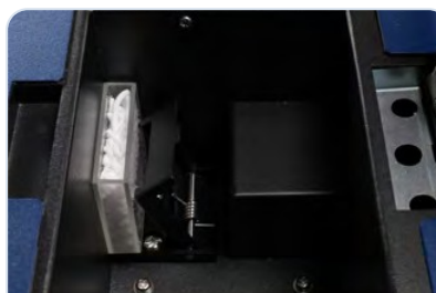
Transmittance chamber with test component and black baffle
