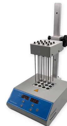
SACO200-1 • one block, 12 needles each with its own valve
