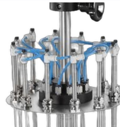
Needle ring • every needle with its own valve and height setting
