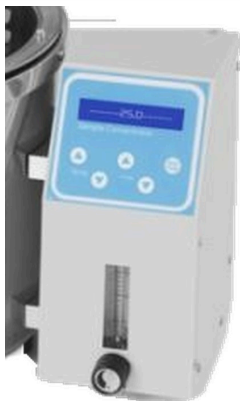
SACO1000 • krmilnik z LCD in merilnikom pretoka
