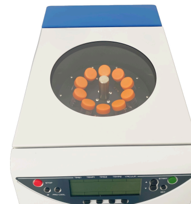
Chamber with rotor seen through the glass window
