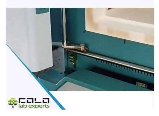
Specially designed door, mounted on a system of levers and springs, by moving it to the side saves space in front devices provide easy sample handlings.
