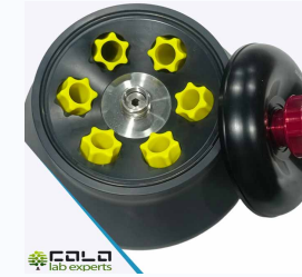
PRO6934 6 × 50 ml sharp / round-bottom rotor 11,000 rpm | 14,400 × g
